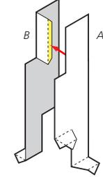
Glue pieces A and B together as shown. Make sure the walls are straight and parallel.
