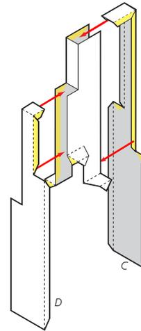
**2** Cut out the tall west wall C and shorter east wall D sections. Fold the flaps and rooftops inwards. Insert the roofs and tabs between the parallel walls A & B. Try to keep the walls and corners as straight and parallel as possible.
