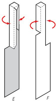
**3** Cut out the north & south side walls E & F. Fold the sides and roofs inwards and glue.
