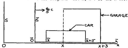
of the front and rear of the garage and let X, X+5 be the  $\overline{x}$ -coordinates of the rear and front of the car respectively. Consider the two events: (i) front of car meets rear wall of garage and (ii) garage doors are slammed. In S, these events have coordinates (i) (X+3,t), (ii) (X,t) (i.e. the events are simultaneous). In S, the events have coordinates (i)  $(X+5,T_1)$ , (ii)  $(X,T_2)$ . The transformation equation  $t = \beta(T+u\overline{x}/c^2)$  applied to these events yields
