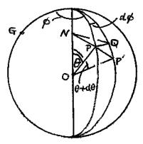
P has colatitude  $\theta$  and longitude  $\phi$ . P' has coordinates  $(\theta+d\theta,\phi+d\phi)$ . PQ is a parallel of latitude with centre N. Since PN =  $\sin\theta$ , PQ =  $d\phi\sin\theta$ , P'Q =  $d\theta$ . To the second order of infinitesimals, we have
