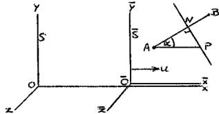
Choose axes in the two frames to be parallel and so that  $\overline{U}$  moves along the x-axis of S with speed u. Then AP is parallel to 0x; denote the angle BAP in S by  $\alpha$ . Also choose the axes so that, in S, the plane BAP is parallel to 0xy.
