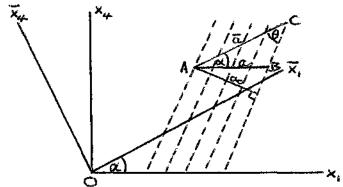
By taking sections of the band parallel to the  $x_1$ ,  $\overline{x}_1$  axes, we obtain the lengths a,  $\overline{a}$ . The rest length  $a_{\sigma}$  is the right-section of the band.
