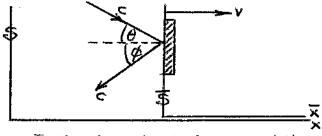
In the frame  $\overline{S}$ , the mirror is stationary, and the angles of incidence and reflection will be equal (say  $\alpha$ ). Thus, photons in the incident and reflected beams will have  $\overline{x}$  velocity components c  $\cos\alpha$ , -c  $\cos\alpha$  respectively. These same photons observed from S will have x velocity components c cos0, -c cos0. The velocity transformation equation requires that
