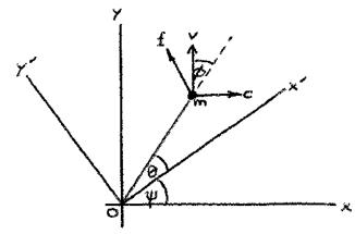
In the inertial frame Oxy, the polar coordinates of the particle are (r,  $\theta+\psi)$  and the polar resolutes of the equation of motion are
