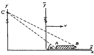
Suppose the bullet AB is attached to the  $\overline{x}$ -axis of  $\overline{S}$  as shown. The camera is placed at C on the y-axis of S. The fixed scale is the x-axis.
